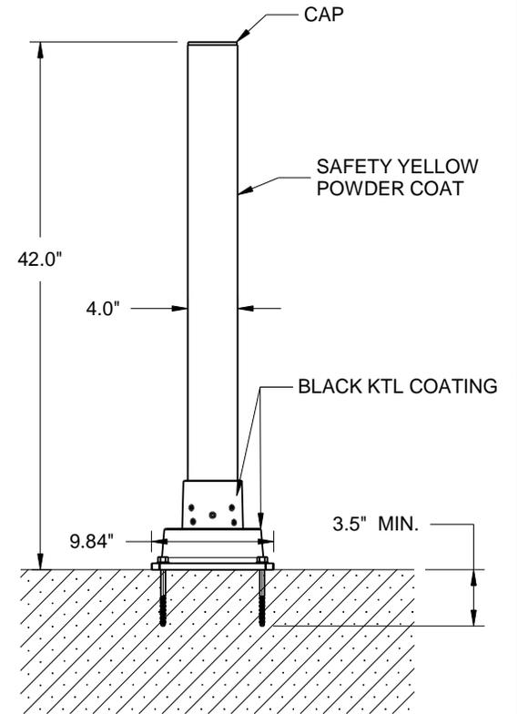
\* MINIMUM FOUNDATION DEPENDS ON LOCAL SOIL CONDITIONS, WEATHER & ENG. REQ'TS
